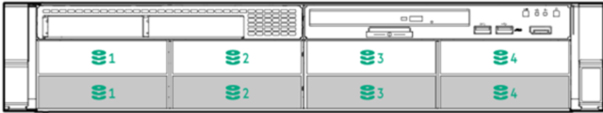
8LFF chassis with Universal media bay and optional 2SFF and optical drive shown
